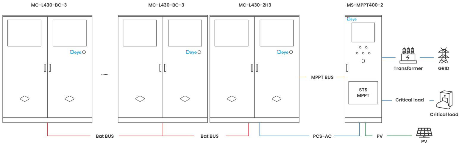
**For ESS on-grid application with solar**
