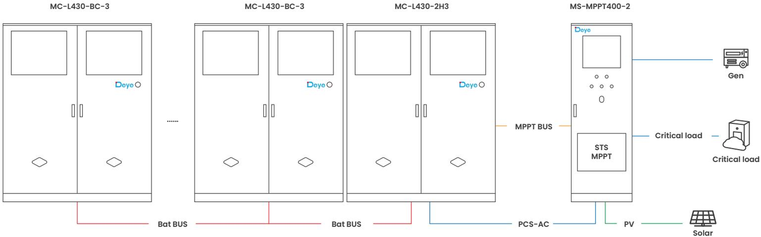
**For ESS off-grid application with solar**
